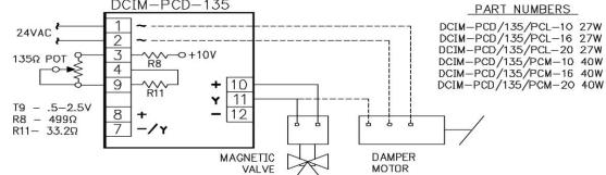
on board) between the 10VDC supply and terminal #3, and (R11 33.2V on board) between terminal #9 and common. The positive leg of the 135V pot connects to terminal #3 and the wiper connects to terminal #9. For a 3 wire pot connect both the
